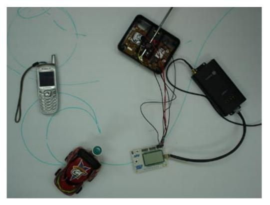
Figure 2: Components for Project 1 (clockwise from top left: cellphone, adapted remote control, cell receiver, ATMEL butterfly, remote control car).
