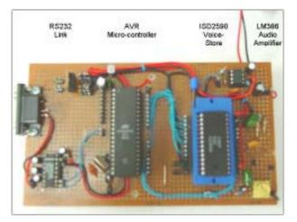
recorded voice feedback. The ISD2590 chip provides programmer to make rapid changes and couple
